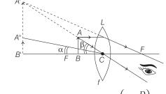
If the image is formed at the near point of eye, then  $m = \left(1 + \frac{D}{f}\right)$
