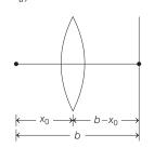
.: Image is formed on screen, hence  $(b - x_0)$  is also the image distance. Image is formed on the screen, so *m* will be negative. **T** 7
