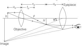
If  $m_o$  and  $m_e$  be the magnifications produced by the objective and the eyepiece respectively, then total magnification of microscope  $m = m_o \times m_e$ .
